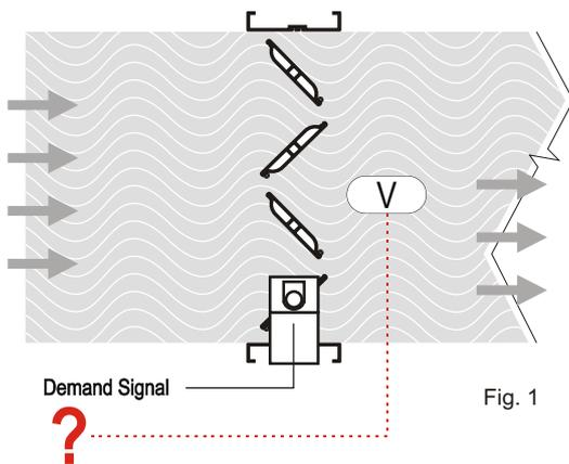
In this type of control (fig. 1), standard motorised volume control damper without airflow measurement is used. Hence the current airflow is dependent on the fluctuation of the inlet or system pressure. That is the reason it is called pressure dependent volume control.
