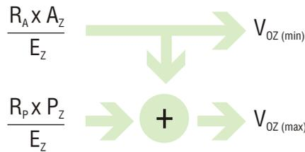
$E_z$  is the zone distribution efficiency, which determines how effectively outdoor air distributes in the zone.
