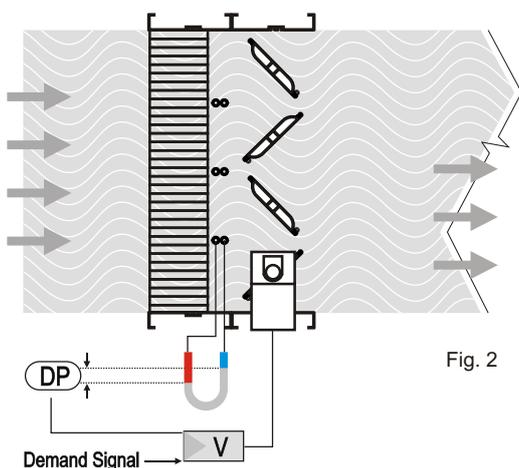
This control (fig. 2), maintains required flow regardless of fluctuation of the inlet or system pressure. Hence it is termed Pressure independent. Variable frequency drives for air handlers can be used with this type of control as it can automatically balance the complete HVAC system.
